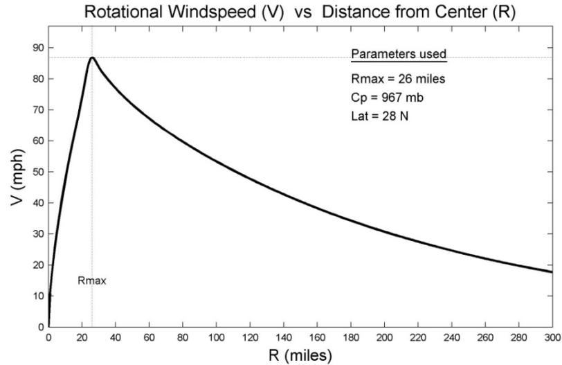
**Figure 45. Symmetric gradient wind profile**
