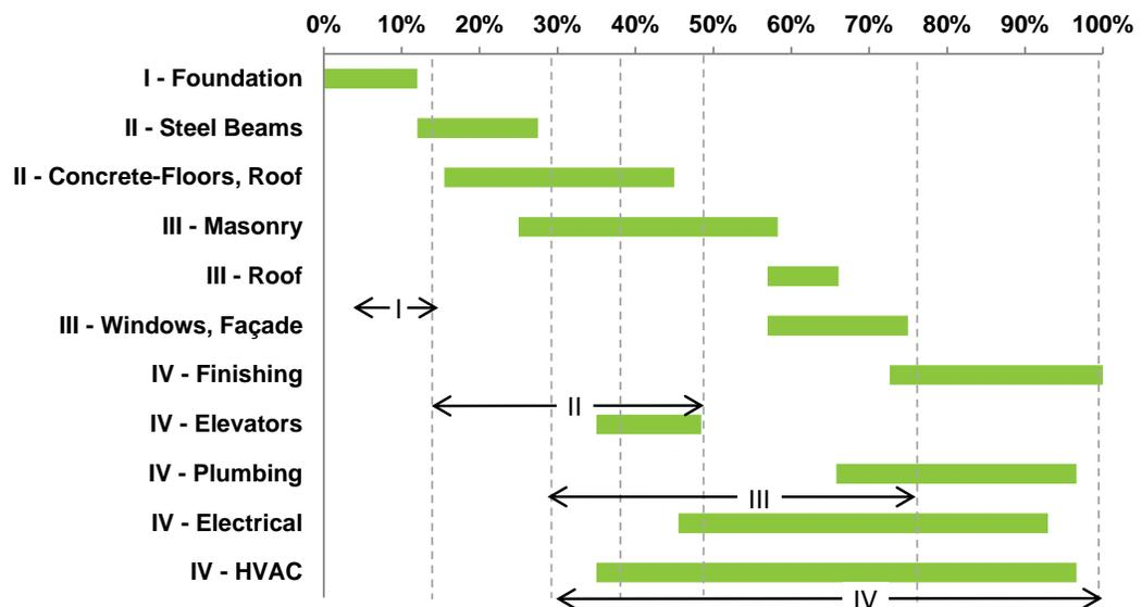
**Figure 77. Duration of some sub-phases for a mid-rise commercial building**
