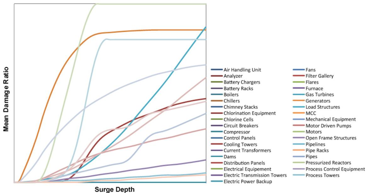
**Figure 104. Storm surge damage functions for industrial facility components**
