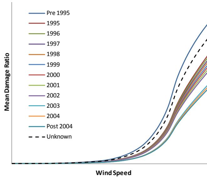
**Figure 66. Year built damage functions for a single-family wood-frame structure in Wilmington, North Carolina**
