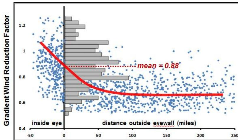
**Figure 44. Mean gradient wind reduction factor calculated by AIR (red line) and corresponding GWRF from Powell et al. 2009 (gray bars)**
