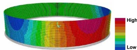
**Figure 91. Distribution of Wind Pressure around a Tank Wall**
