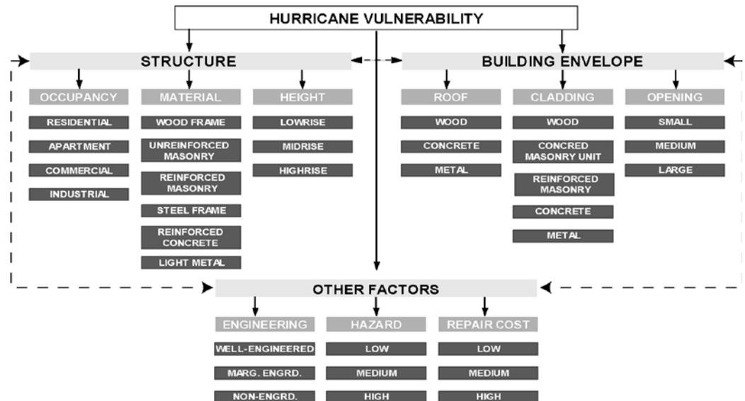
**Figure 58. Component-based vulnerability model for commercial structures**
