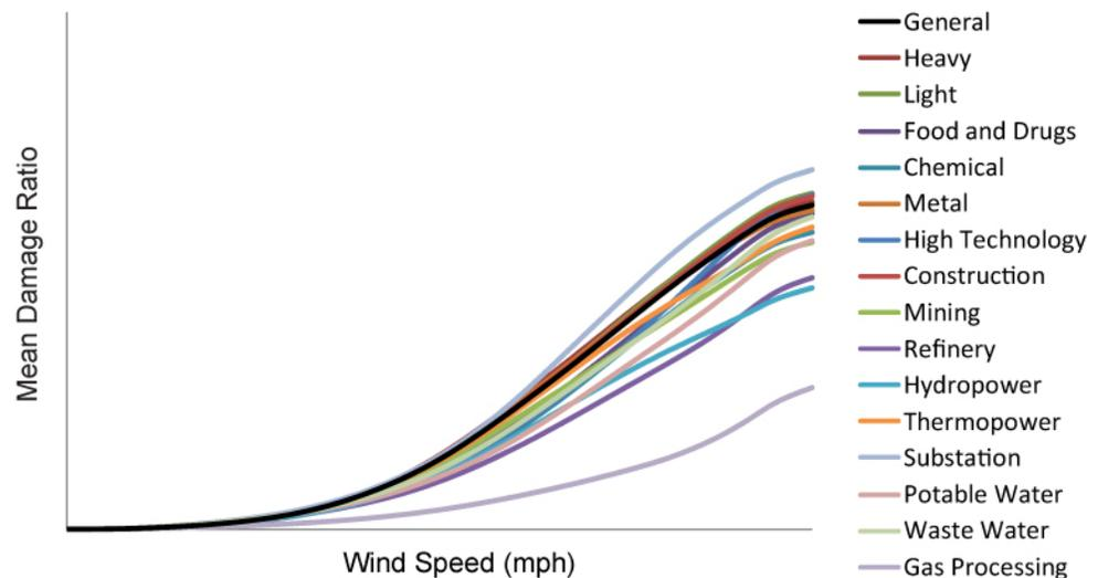
**Figure 105. Industrial facility-level wind damage functions**
