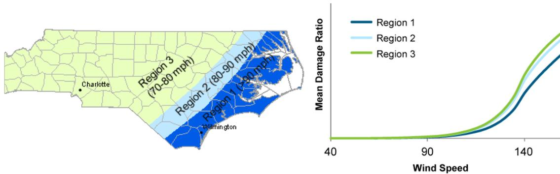
**Figure 64. Vulnerability regions for structures built in 1995-2002 in North Carolina and corresponding damage functions**
