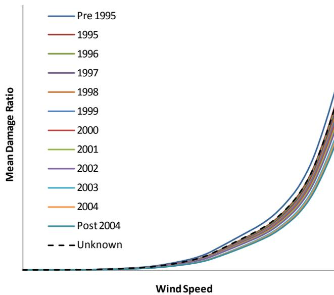
**Figure 67. Year built damage functions for a commercial reinforced-concrete structure in Wilmington, North Carolina**
