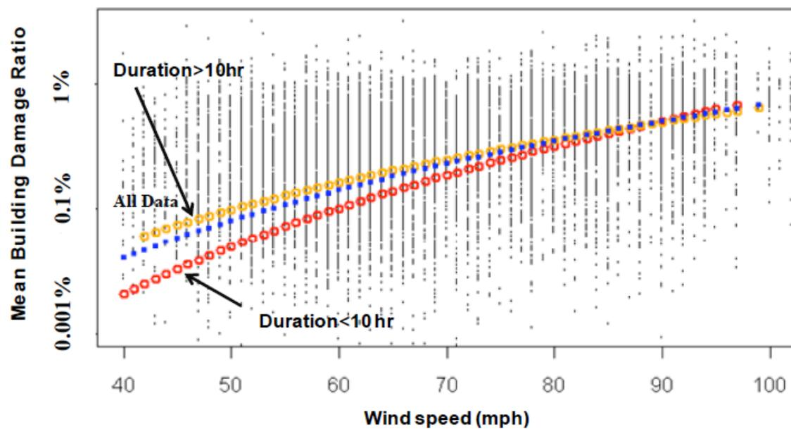
**Figure 61. The effect of wind duration on the mean damage ratio (Source: Jain et al. 2009)**
