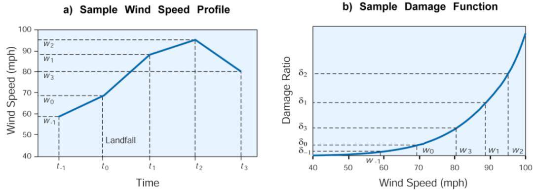
**Figure 60. (a) Sample wind speed profile and (b) corresponding damage ratios**
