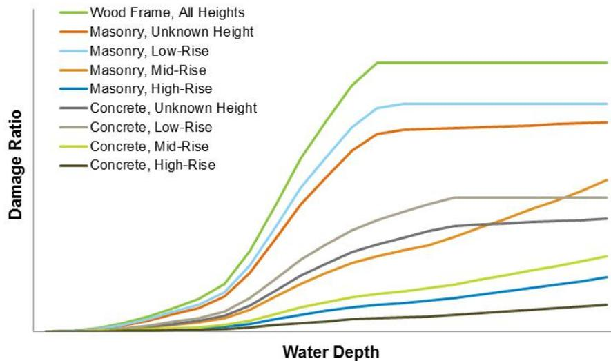
**Figure 68. Storm surge damage functions for different height and construction categories, general commercial occupancy**
