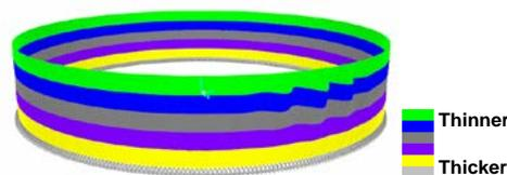
**Figure 92. Deflection of Tank Wall at Onset of Elastic Buckling (Colored Bands Represent Different Levels of Tank Shell Thicknesses)**
