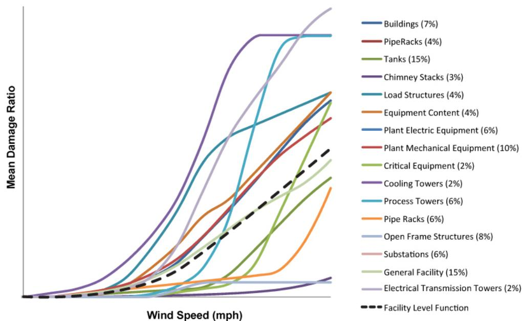
Figure 101. Wind damage functions for a sample industrial facility
