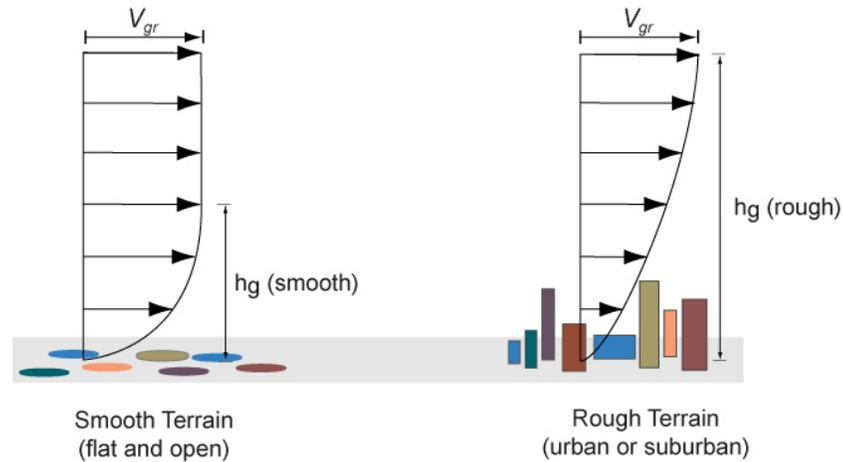
**Figure 46. Terrain effects on wind-velocity profiles (adapted from Cook, 1985)**
