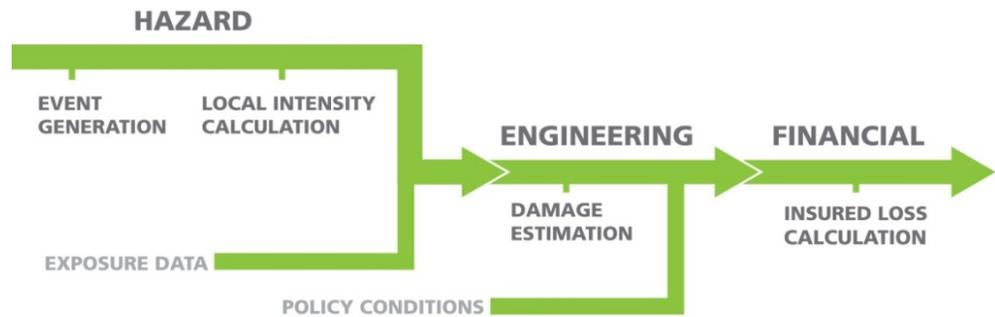
**Figure 12. Components of the AIR Hurricane Model for the United States**
