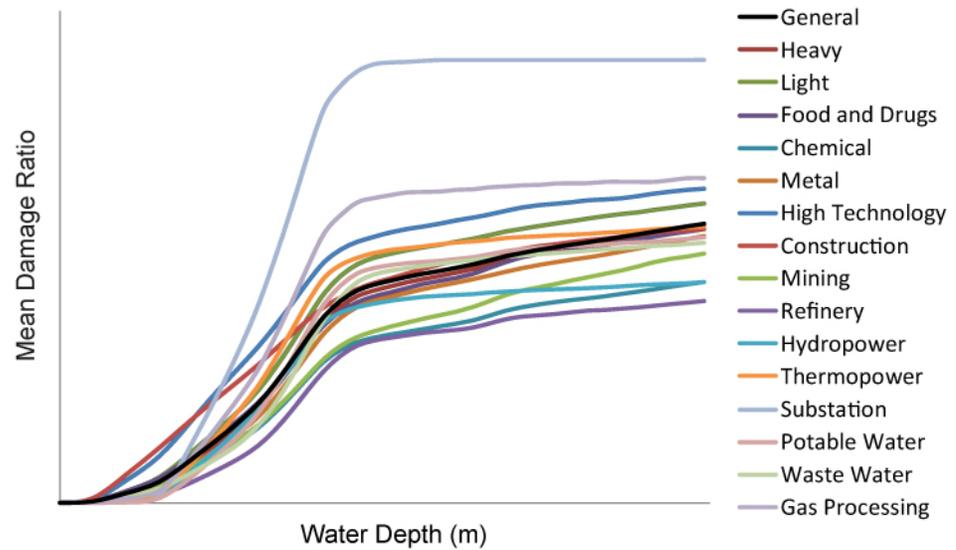
**Figure 106. Industrial facility-level storm surge damage functions**
