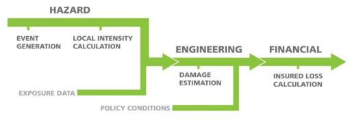
Figure 12. Components of the AIR Hurricane Model for the United States
