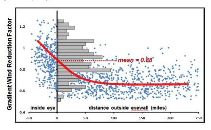
Figure 44. Mean gradient wind reduction factor calculated by AIR (red line) and corresponding GWRF from Powell et al. 2009 (gray bars)
