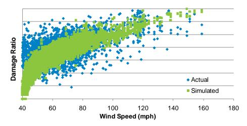
Figure 85. Observed and modeled damage ratios at different wind speeds, Coverage D
