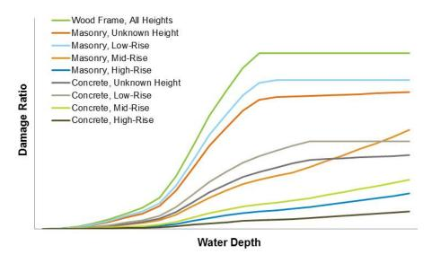
Figure 68. Storm surge damage functions for different height and construction categories, general commercial occupancy
