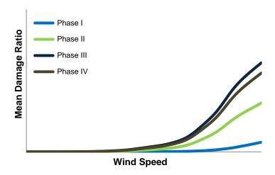
Figure 81. Wind damage functions by building phase for an engineered midrise commercial building
