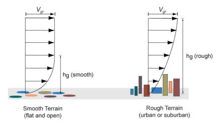
Figure 46. Terrain effects on wind-velocity profiles (adapted from Cook, 1985)
