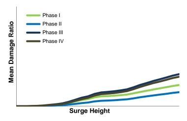
Figure 82. Surge damage functions by building phase for an engineered mid-rise commercial building
