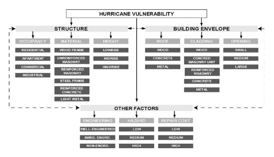
Figure 58. Component-based vulnerability model for commercial structures
