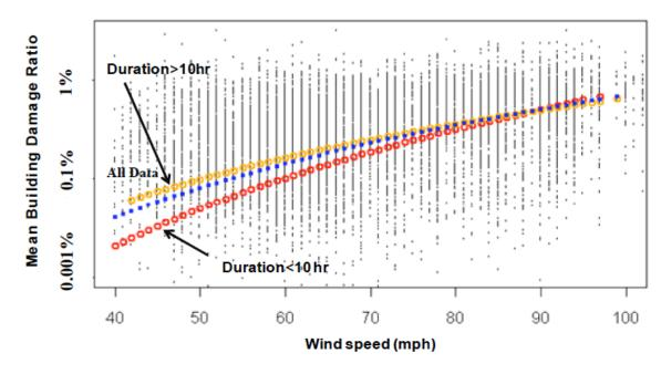
Figure 61. The effect of wind duration on the mean damage ratio (Source: Jain et al. 2009)
