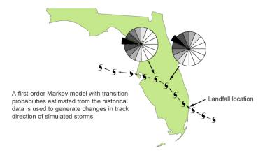
Figure 30. Generation of the model's storm track
