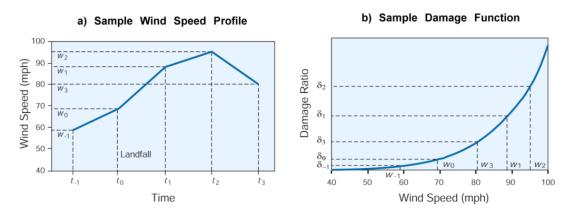
Figure 60. (a) Sample wind speed profile and (b) corresponding damage ratios
