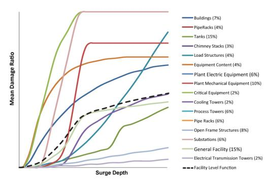
Figure 102. Storm surge damage functions for a sample industrial facility
