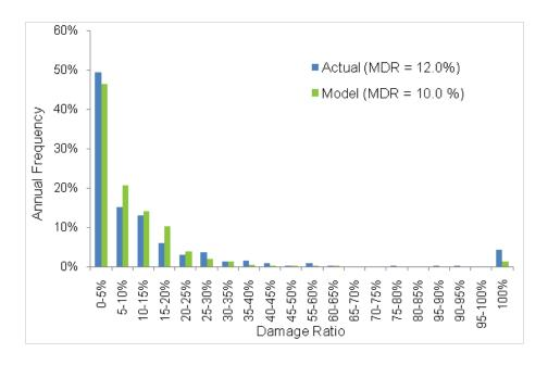
Figure 87. Observed and modeled uncertainty around the mean damage ratio
