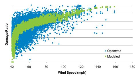
Figure 83. Observed and modeled damage ratios with wind speeds, Coverage A
