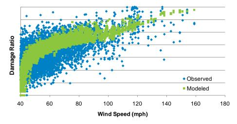
Figure 84. Observed and modeled damage ratios at different wind speeds, Coverage C
