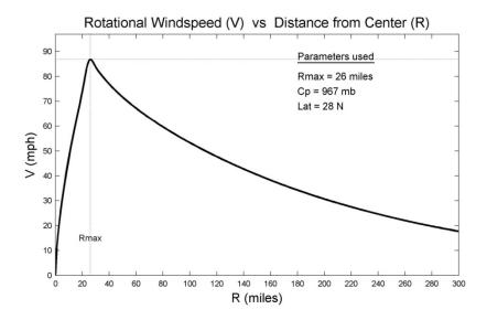
Figure 45. Symmetric gradient wind profile
