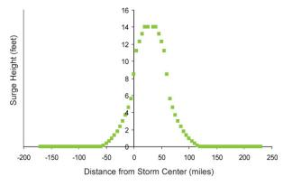
Figure 32. Surge profile for sample storm with central pressure of 953 mb and Rmax of 30 miles
