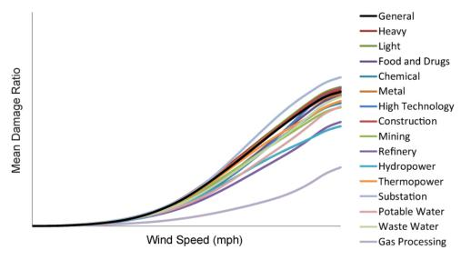
Figure 105. Industrial facility-level wind damage functions
