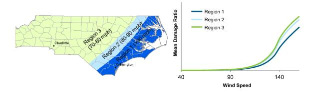
Figure 64. Vulnerability regions for structures built in 1995-2002 in North Carolina and corresponding damage functions
