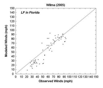
Figure 53. Observed and modeled wind speeds (mph) for Hurricane Wilma
