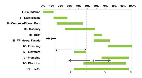
Figure 77. Duration of some sub-phases for a mid-rise commercial building
