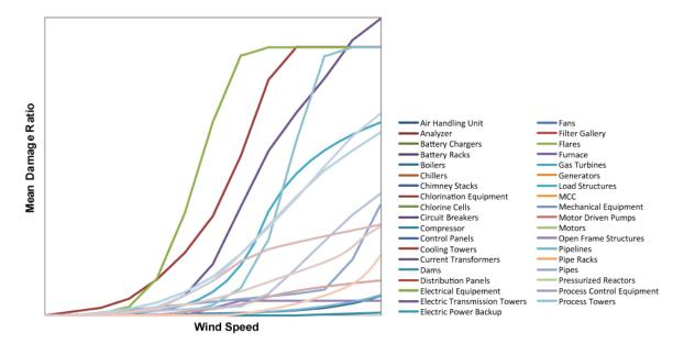
Figure 103. Wind Damage functions for industrial facility components
