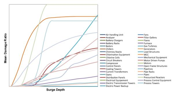
Figure 104. Storm surge damage functions for industrial facility components
