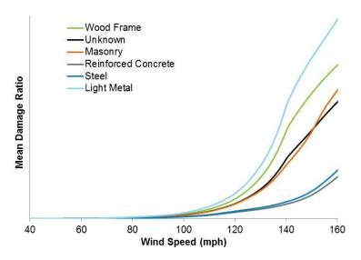
Figure 59. Wind damage functions for selected construction classes
