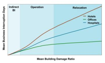
Figure 73. Impact of factors determining business interruption downtime varies with occupancy and severity of building damage
