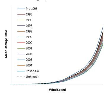
Figure 67. Year built damage functions for a commercial reinforced-concrete structure in Wilmington, North Carolina
