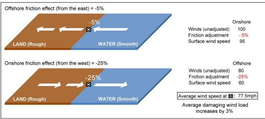
Figure 49. Schematic of the effect of directionality on friction
